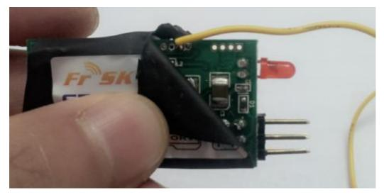
6. Power supply GPS sensor via S.PORT, connection the +, - to Battery
