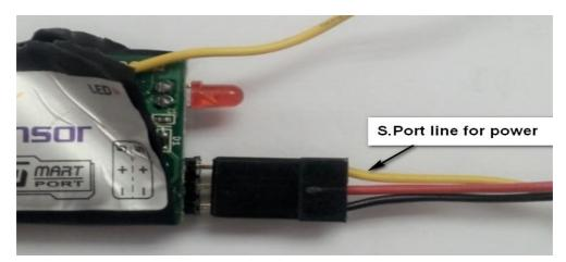
7. The other end of the wire is connected to Frsky HUB in the correct position Please be close attention do not connected in wrong pin!!!
